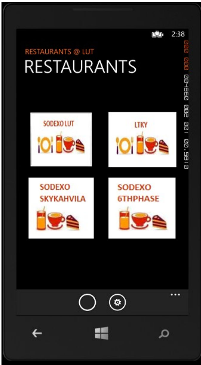
Illustration 1: Main page of the application. There are four clickable restaurant buttons and two buttons ("eat" and "settings") on the application bar. Note: "eat" button (the empty circle) doesn't have a proper icon and the application doesn't have any settings just yet.
