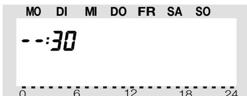
Use the selection wheel to set the desired minutes, and confirm your setting by pressing the “PROG” key.
