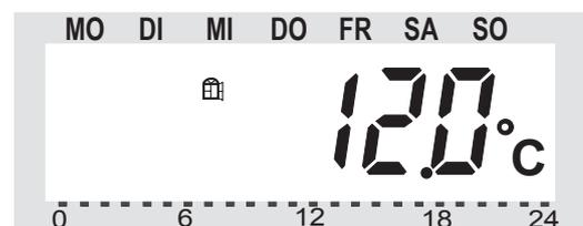
Use the scroller to set the 'Window open' temperature you require. To confirm briefly press the '☾ ☀' button.
