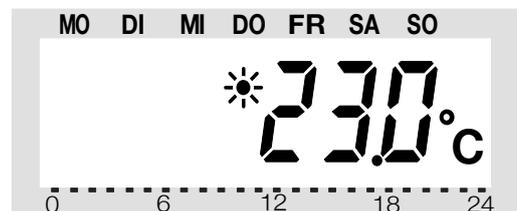
Use the scroller to set the desired comfort temperature. To confirm briefly press the '☾ ☀' button.
