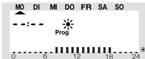
If you set the second comfort temperature time to „--:--“ the setting of the second lowering temperature time is irrelevant, since no data are changed. In all, you may set two periods of time for comfort temperature, e.g. from 6.00 to 9.00 hrs and from 16.00 to 23.00 hrs.
