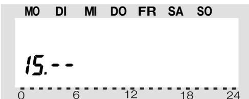
Use the selection wheel to set the desired day, and confirm your setting by pressing the „PROG” key.
