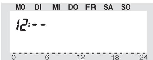
Use the selection wheel to set the desired hour, and confirm your setting by pressing the “PROG” key.
