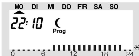
Use the selection wheel to select the time when control of the lowering temperature is to be started.
