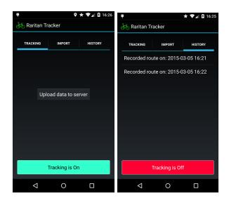
The graphical interface of the application consists of three tabs, Tracking, Import and History. The actual tracking is happening in the first tab, on the click of the button "Tracking is Off" the colour and the text will be changed to "Tracking is On", and in the background a couple of things are triggered.
