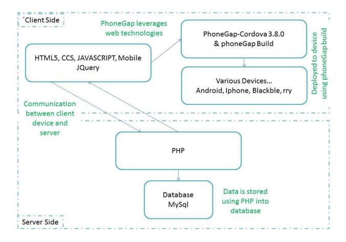
Picture 2 Architecture of front and back-end of ZEROS
